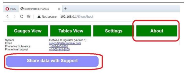
In order to view the information on the regulator's website, users run an internet explorer on any platform, and type the local IP address in the address bar. When a gauge is grayed out, it means that there is no corresponding input. Field Reduction Switch buttons "FRS+" and "FRS-" appear when the PRO X regulator is in charging mode. Remote Support is enabled by clicking "Share Data with Support" button in the "About" section of the website.
